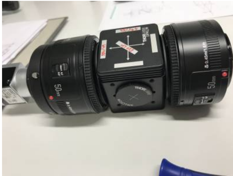
Figure 5: Completed Filter Cube with camera and Objective 1 on the left and Objective 2 on the right.
