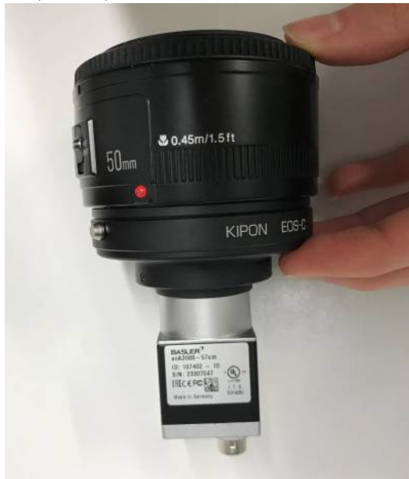
Figure 3: Camera (bottom) attached to the adaptor and tube lens.
