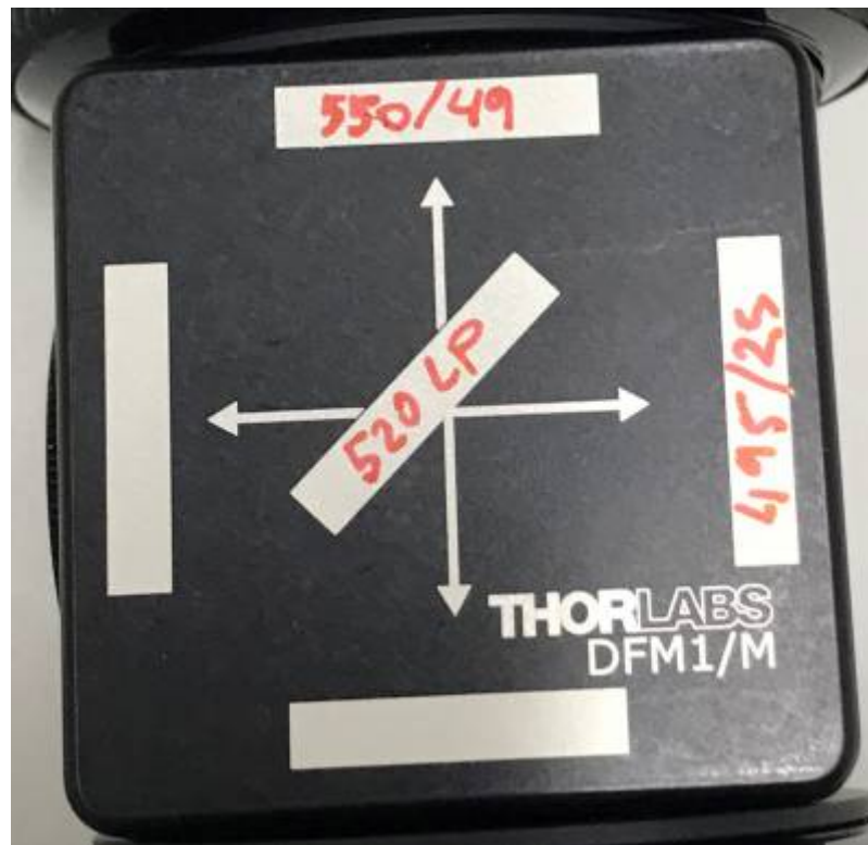
Figure 4: Outside portion of the Filter Cube showing the orientation of the filters inside. The white rectangles along the edges are the optical filters, while the slanted rectangle in the center is the dichoric mirror.
