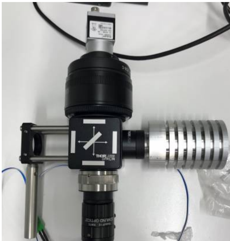
Figure 7: Fully assembled microscope optics. On the left of the Filter Cube, the metal poles and cage plate (black) are used to fix the optics to the microscope stand.
