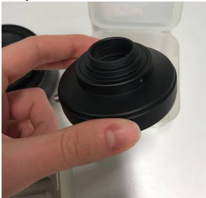
Figure 1: EOS to C-mount adaptor.
